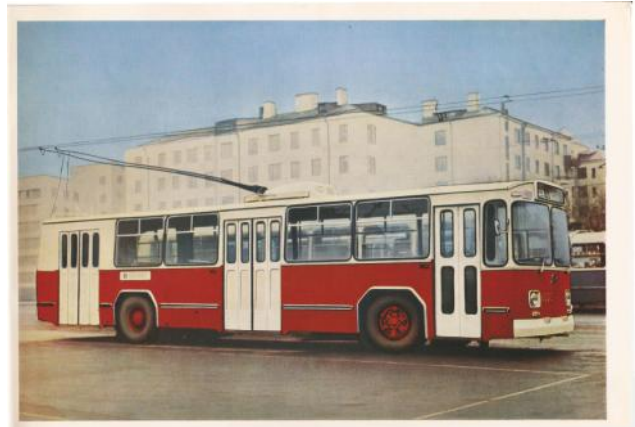
ZIU-9: In typical Russian fashion, passengers board at the rear & pass a seated conductor. (ZIU)
